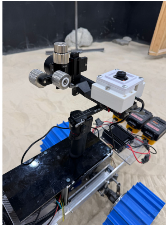
Figure 14: Fisheye Camera mounted on Mechanical Gimbal
