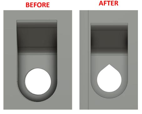
Teardrops were used to ensure optimal vertical holes with minimal support
