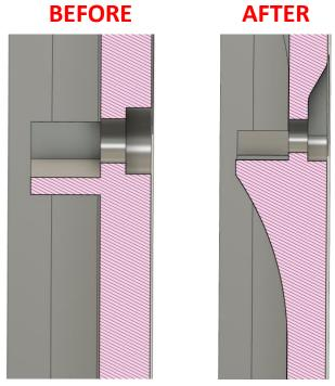
Horizontal overhangs were eliminated by gradually reducing the overhang angle, thereby reducing support material
